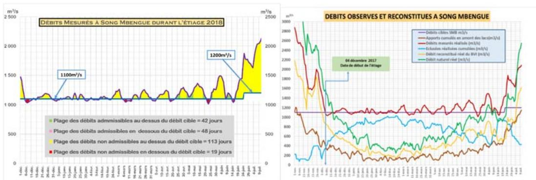
In the dry season of 2018, the measured flow rate of Song Mbengué is 700 m<sup>3</sup>/s, which can meet the water impoundment requirement 70% of the time. The average flow rate in this period is set at 1,192 m<sup>3</sup>/s, which is 8% higher than the target value.
