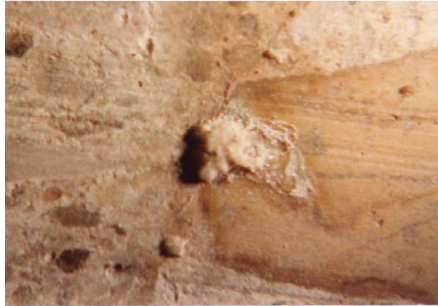
Fig. 4.16 - Formation silica gel at the interface between aggregate particle and cementitious matrix.
