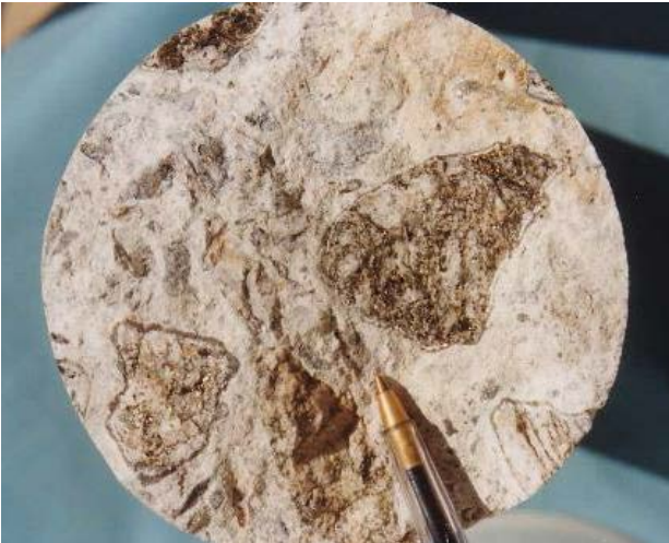
Fig. 4.14 - Dark rims surrounding reactive particles in a dam concrete core.
