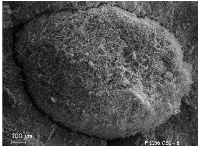
Fig. 4.22 - Massive-textured secondary ettringite crystals in a concrete pore
