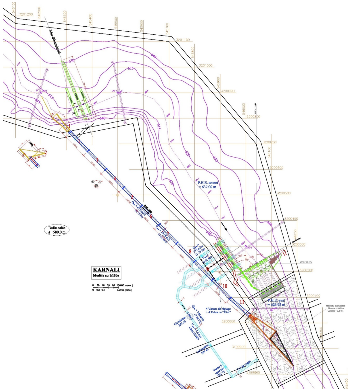
Fig. 3.5 Plan view of the Karnali hydroelectric scheme
