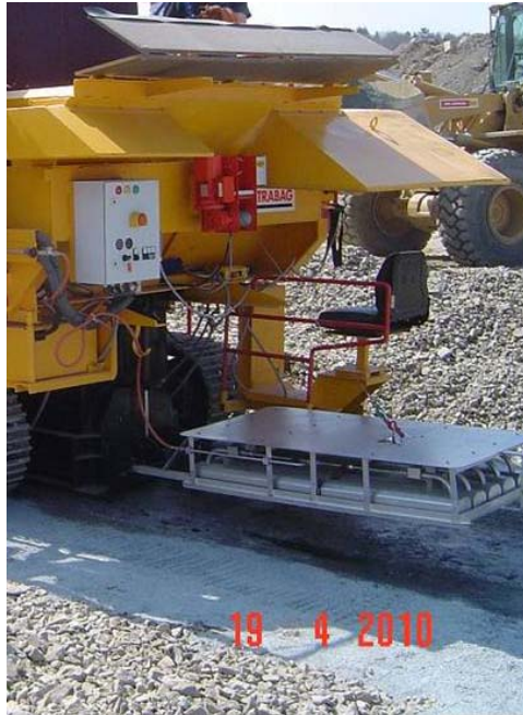
Figure 5.19 Infrared heater in front of core paving machine
