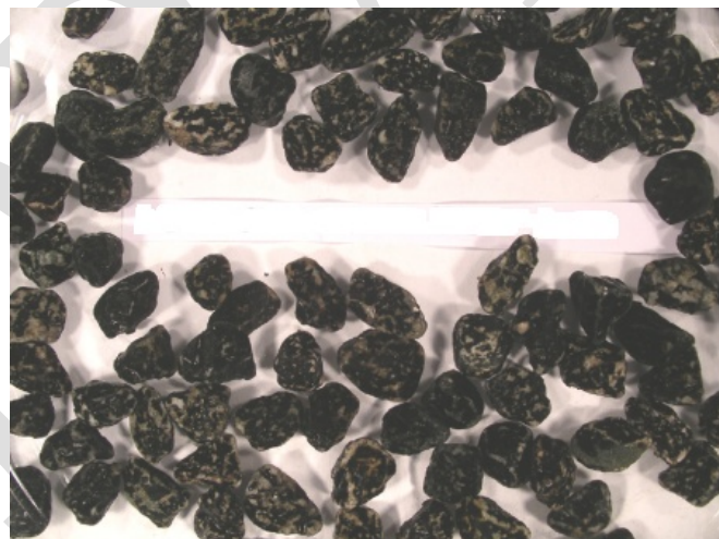
Figure 6.2 Adhesiveness after 72h water storage with bonding agent
