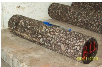
Figure 5.9 Drilled and sliced samples from the AC core
