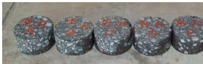
Figure 5.9 Drilled and sliced samples from the AC core
