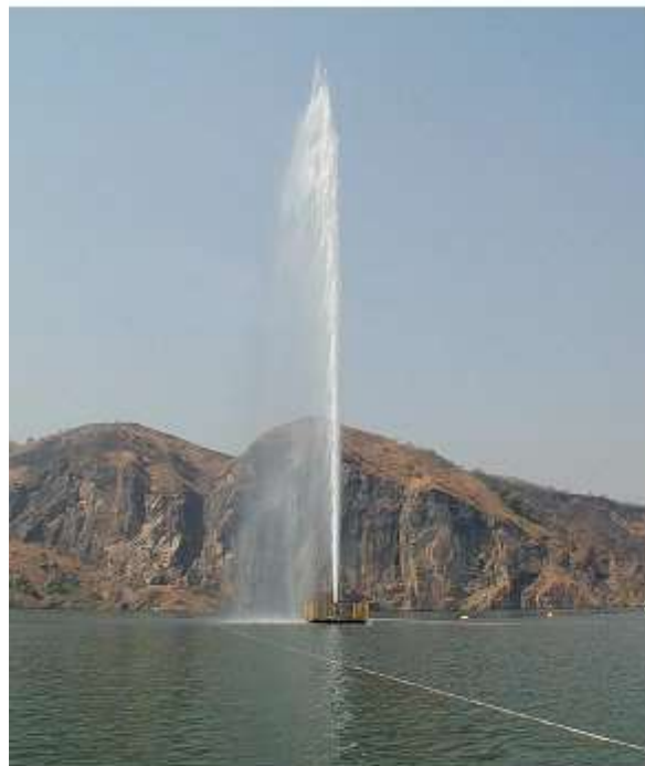
Figure 3-11: Degassing pipe in action
