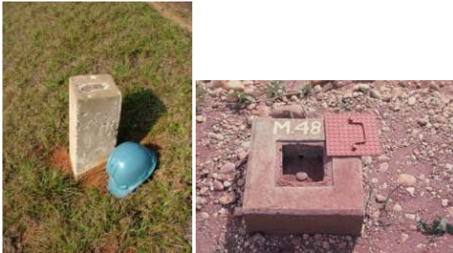
Fig. 6.7 – Two types of benchmarks installed at the downstream slope.
