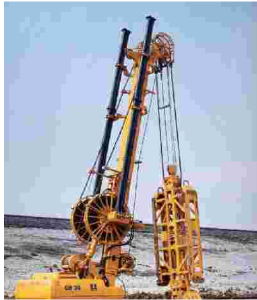
Fig. 3.6 Hydraulic grab (Bauer type 1998)
