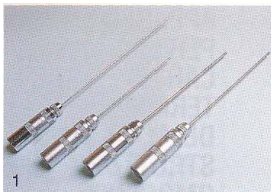
Fig. 6.8 – Needle probes for thermal tests on concrete specimens in laboratory
