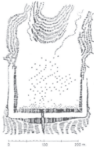
Fig. 69 Layout of the 8 m high Karakuyu dam in Uzunyayla, with a total crest length of 400 m, from 13 century B.C.
