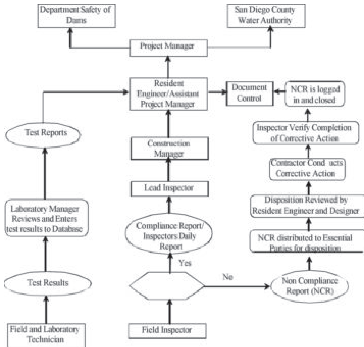
Fig. 15 Testing and Inspection Report Distribution
