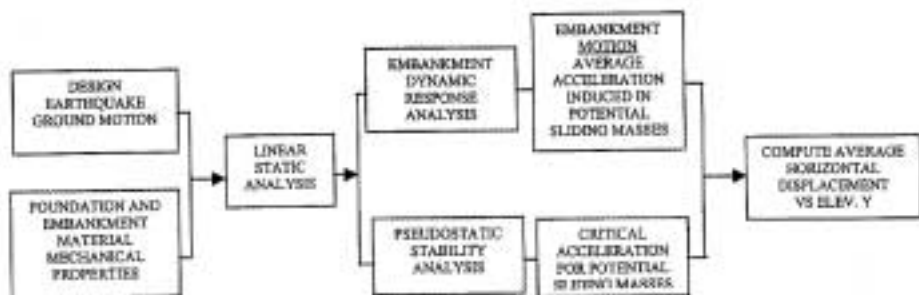
Flow chart representing the main steps of seismic analysis using equivalent linear approach and Newmark procedure
